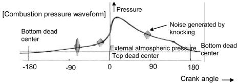
(This crank angle will be 720 degrees with 4 cycle engine)
