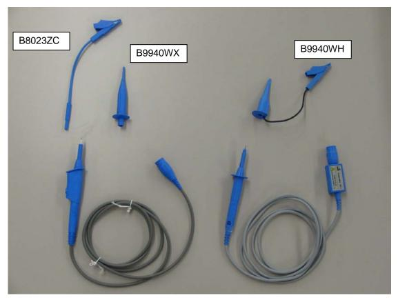
The new 700929 has two parts, Safety pulg-on clip(B9940WX) and Safety  $clip\ lead(B8023ZC)$ . The old 700929 has only one part, Pincher Tip(B9940WH) which has a ground lead .
