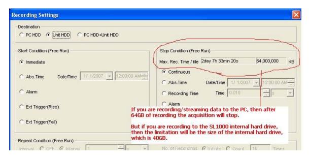
Also, the dead time between file creations (segmented) is zero. There is no data loss. Since the SL1000 allocates enough memory, no data is lost between closing a file and opening a new one.
