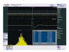
The shape of the curve doesn't indicate the actual pulse envelope, but the output of the photo detector, which, although orders of magnitude slower, still corresponds to the impulse intensity. The list in the lower right indicates maximum values,
