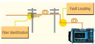
The AQ7275 OTDR can be ordered with a visible light source. This source can be used to identify which fiber you are working on. It can also be used to check for sharp bends in the fiber. The light is pulsed on and off at a rate of 2 Hz times per second. Light generated by this source will escape from sharp bends and breaks in jacketed or bare fibers, as well as poorly mated connectors. It
