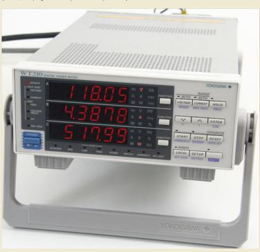
We've also beefed up our lab equipment by stepping up to a Yokogawa WT210 power meter. The Extech unit we've used in the past would occasionally return an obviously erroneous value, and for that reason, the Extech hasn't been sanctioned for use with SPECpower\_ssj when the results are to be published via SPEC. The WT210 is a much more accurate meter that meets with SPEC's approval and integrates seamlessly with the SPECpower\_ssj power measurement components.
