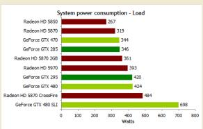
Well, that's not very good. At idle, the GTX 470's power draw isn't too scary, but the GTX 480 pulls more juice than the dual-GPU Radeon HD 5970. Two idle GTX 480s in SLI draw just 20W less than a Radeon HD 5850 does while running a game.
