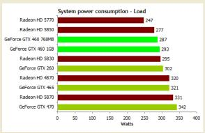
Overall, the new GeForces look quite decent on power draw. Interestingly, the Radeon HD 5850 draws less power under load than either flavor of GTX 460, yet the slower Radeon HD 5830 draws more. There's a simple reason for that: the GPU on 5830 has more units disabled, but it also has a higher clock speed than the 5850. Higher clock frequencies increase power draw, and higher voltages are often required to reach them. With a larger board and higher clocks the 5830 isn't particularly efficient.
