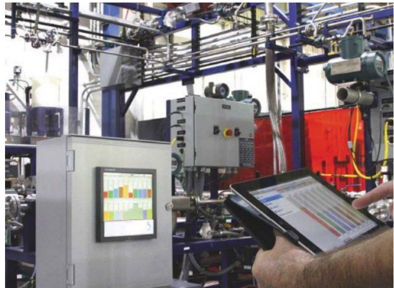
Figure 1: Multi-touch technologies implementation in tablet PC and data acquisition enables remote control and data analysis through Bluetooth or WiFi.
