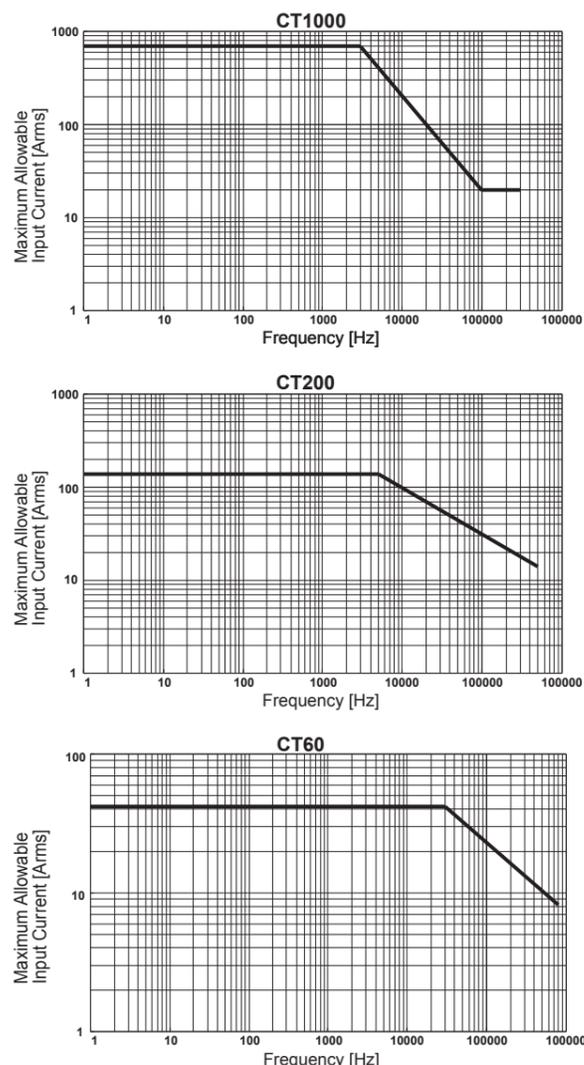
Figure 4. Derating of Primary Current by Frequency
