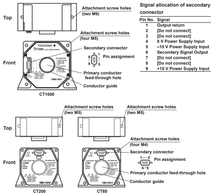
Figure 1. Names of Parts and Pin Assignments
