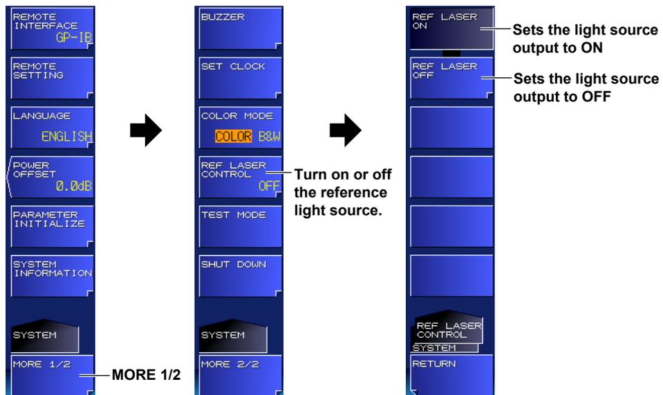
4. Press the **REF LASER ON** or **REF LASER OFF** soft key.
