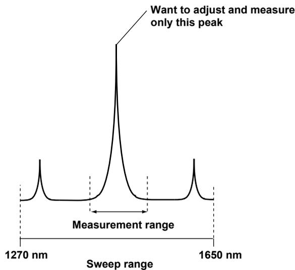
Peaks outside the measurement range will not be detected. The spectrum waveform will consist only the peaks within the limit range (measurement range). In this situation, scaling is also limited within the range.
