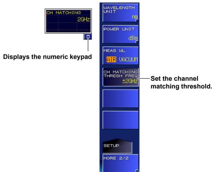
4. Enter the threshold using the arrow keys or numeric keypad.
