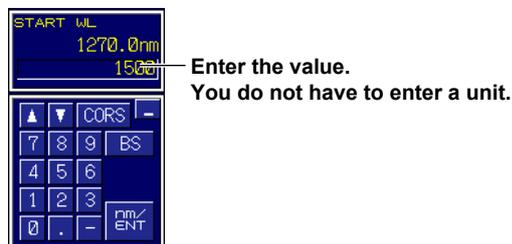
5. Enter the start wavelength using the arrow keys or numeric keypad.
