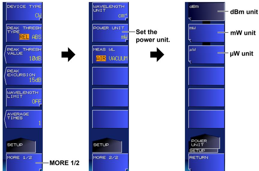
4. Press the **dBm**, **mW**, or **μW** soft key.
