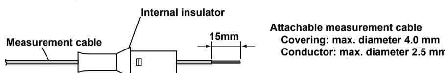
2. Insert the tip of the measurement cable into the plug. Fasten the measurement cable in place using the supplied hexagonal wrench.
