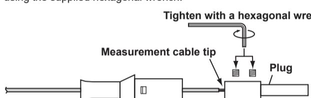
3. Insert the plug into the internal insulator.
