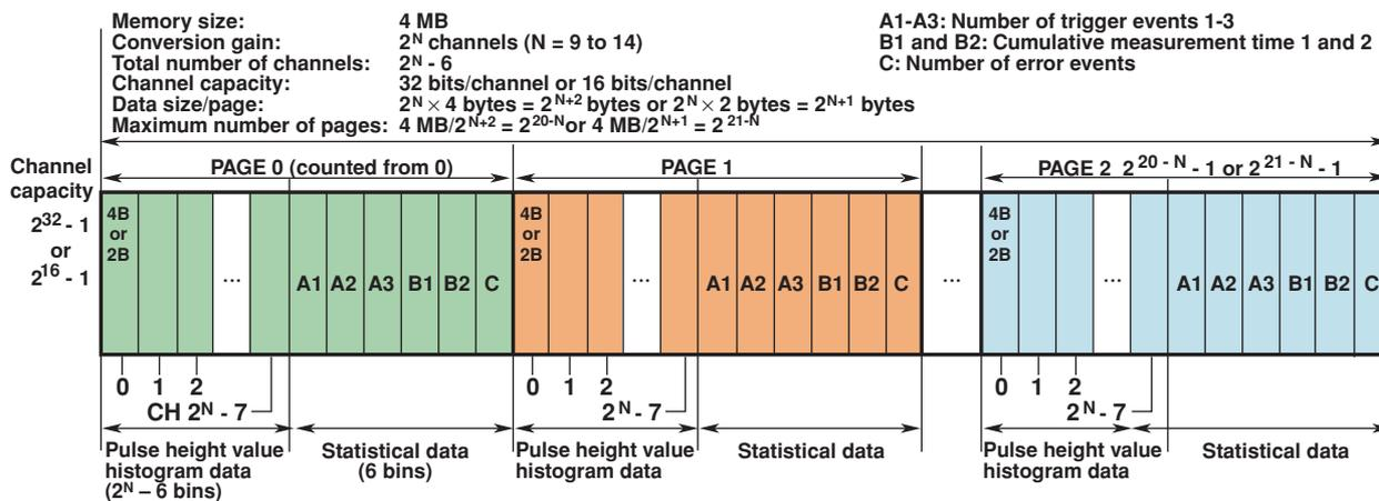
The value N in the above figure is the bit-converted values of the total number of AD channels in the following table.
