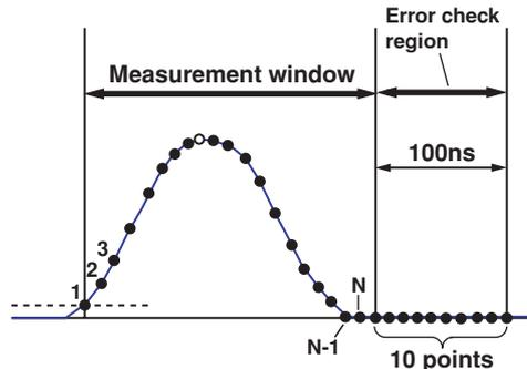
If a signal having two peaks in the measurement window is applied, the larger of the two peak values is determined to be the peak value of the event, and the other peak value is discarded.
