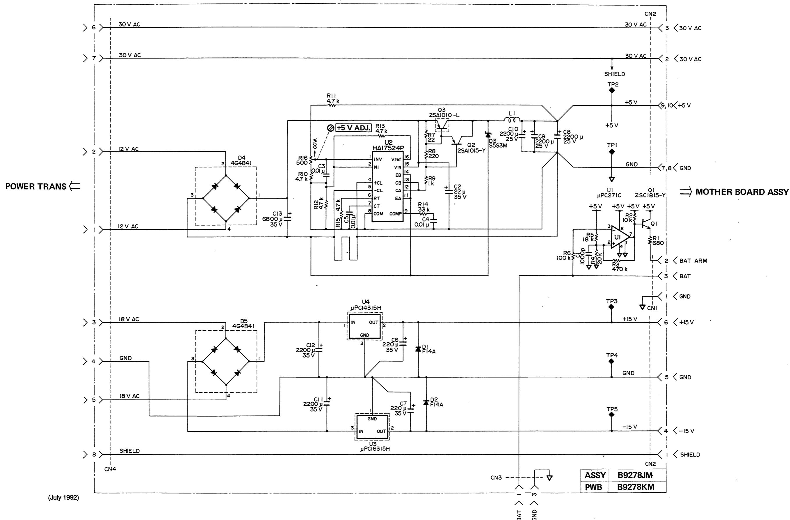
Figure 5-9a. Power Supply Board Ass'y (for Model 2533E31): B9278JM Schematic Diagram.
