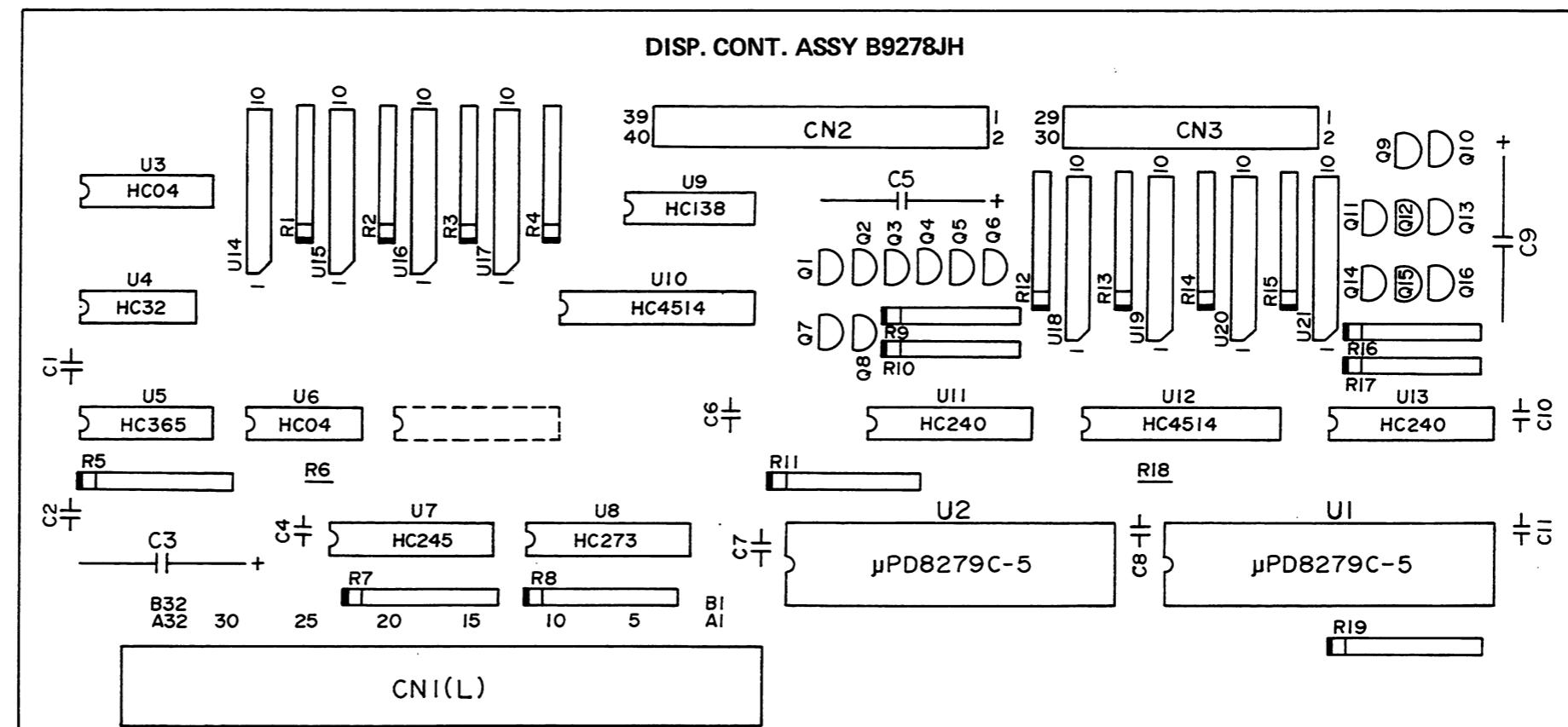
Figure 5-7b. Display Control Board Ass'y: B9278JH Components Location Diagram.
