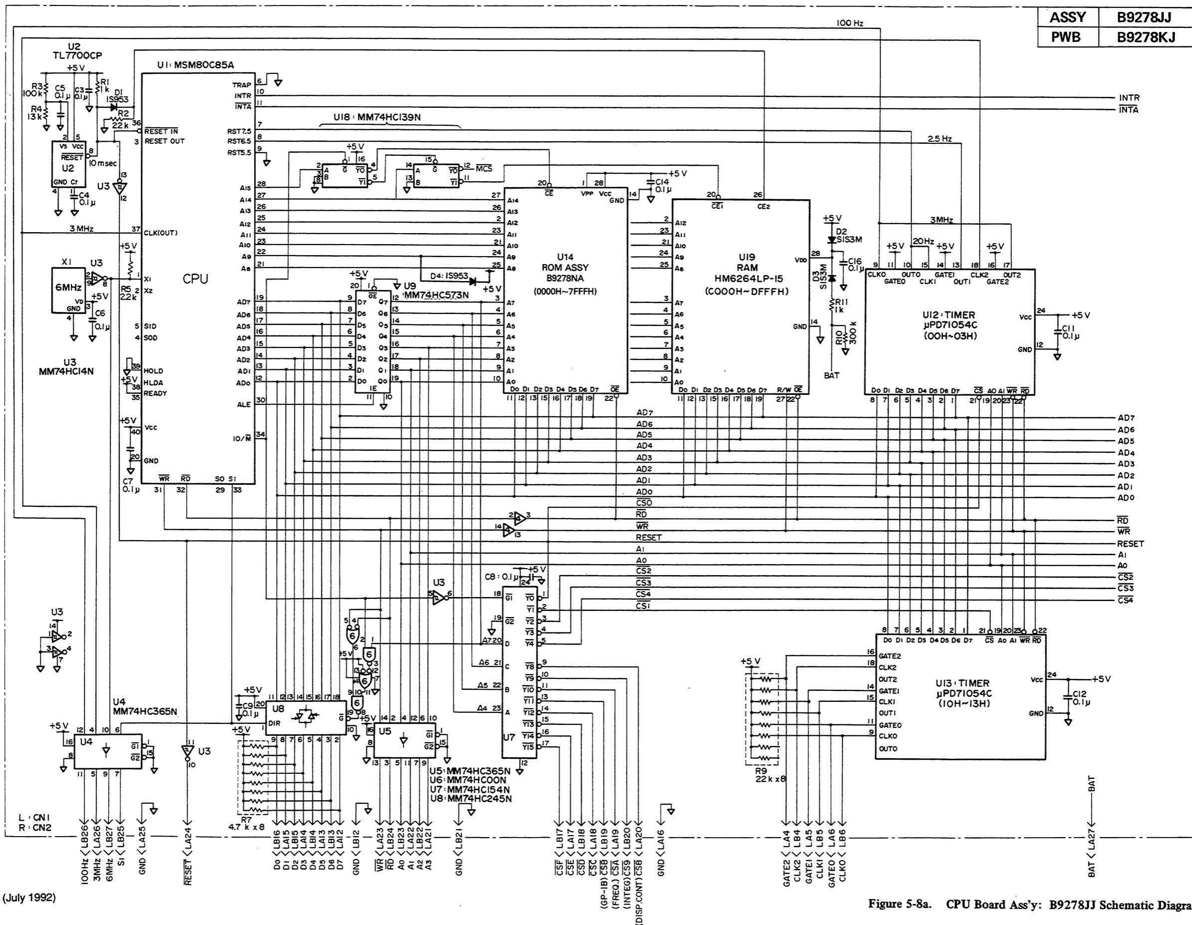
Figure 5-8a. CPU Board Ass'y: B9278JJ Schematic Diagram (1/2).
