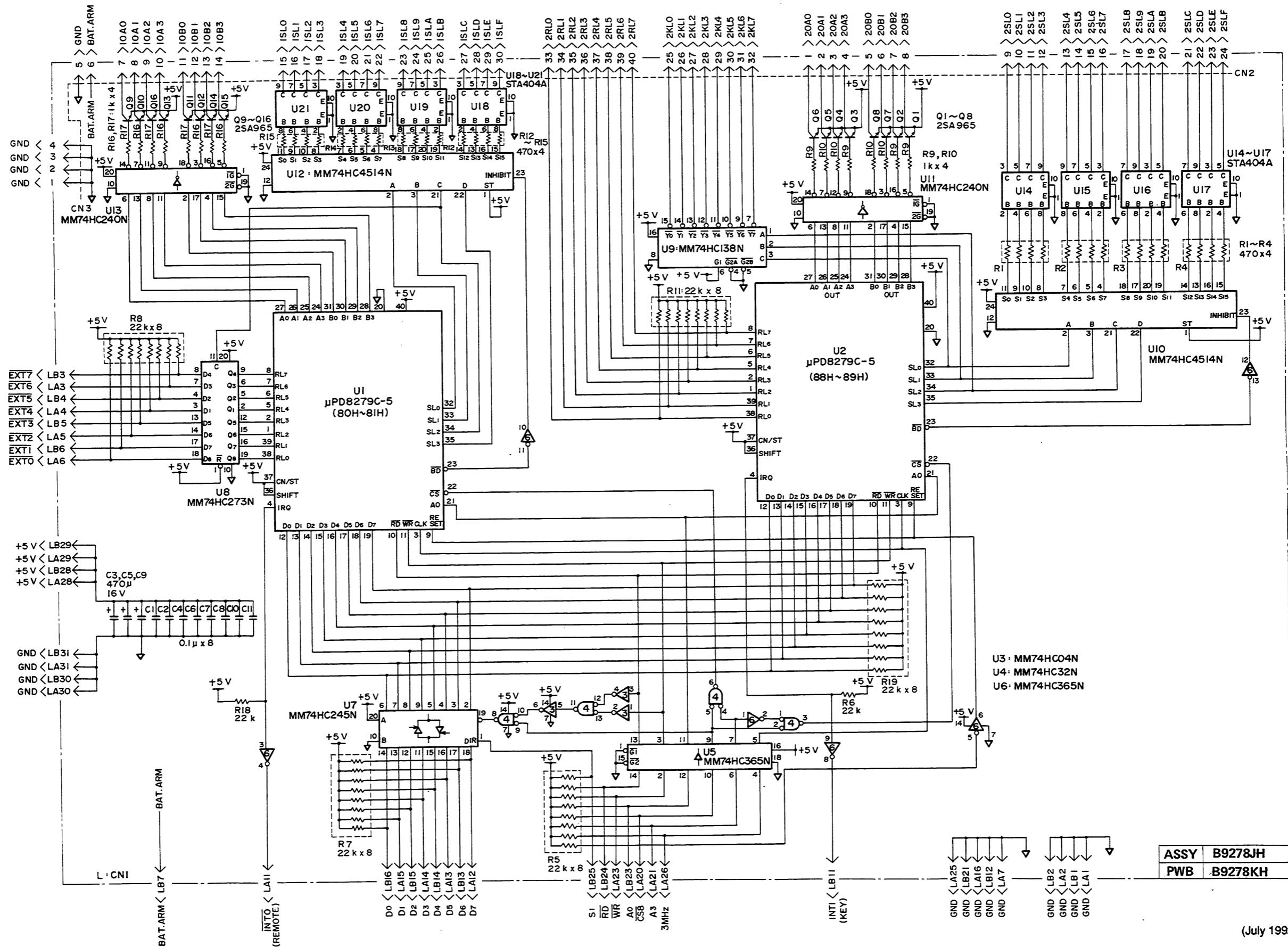
**Figure 5-7a.** Display Control Board Ass'y: B9278JH Schematic Diagram
