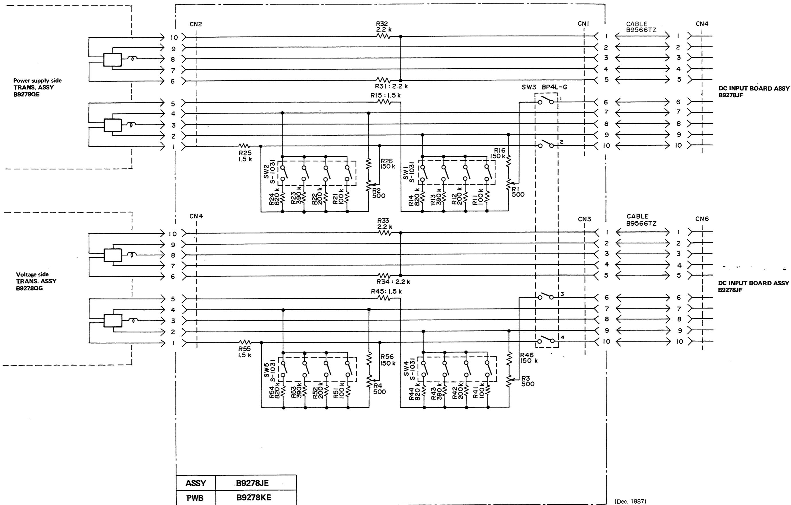
Figure 5-3a. Sub Board Ass'y (for Model 2533E41): B9278JE Schematic Diagram.
