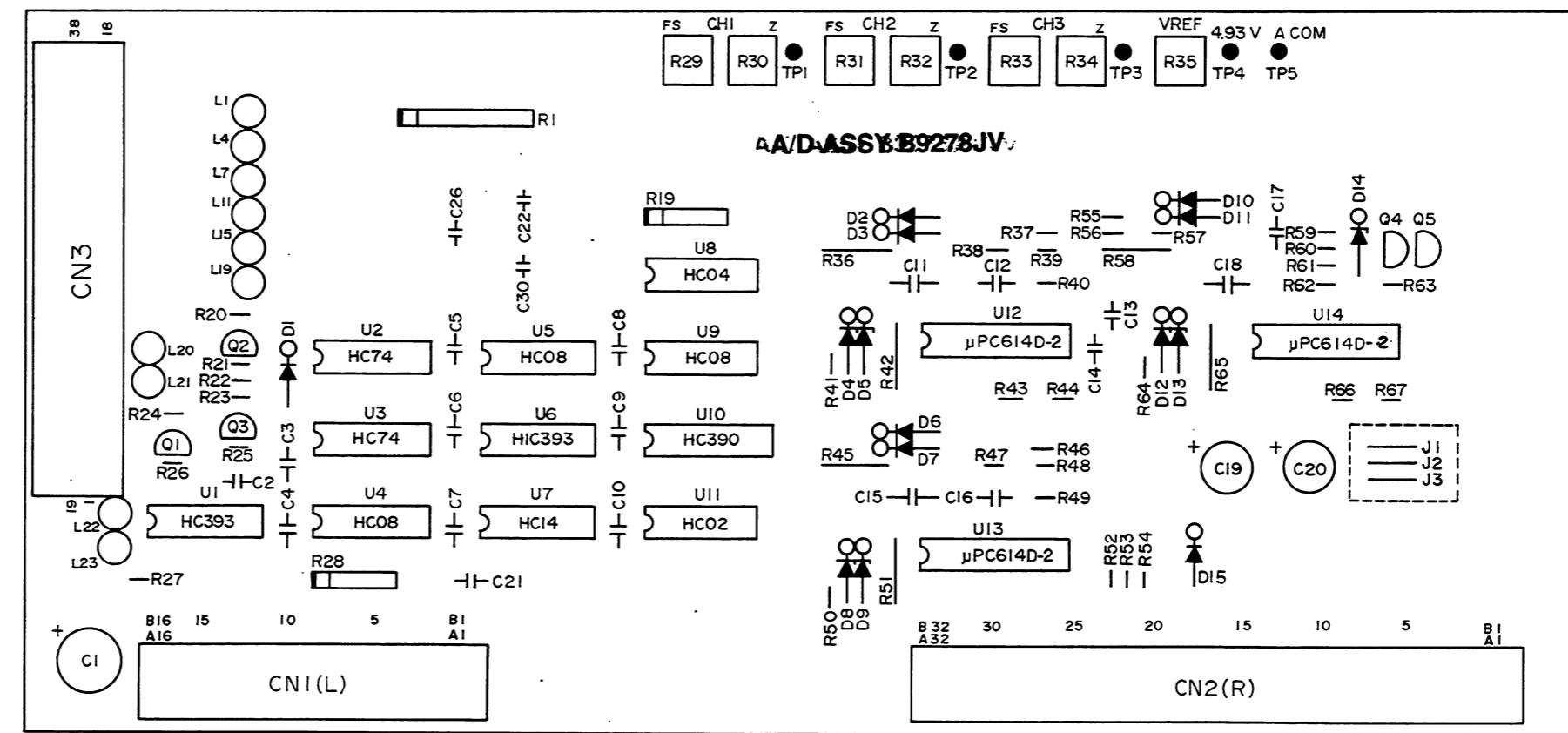
Figure 5-6b. A/D Converter Board Ass'y: B9278JV Components Location Diagram.
