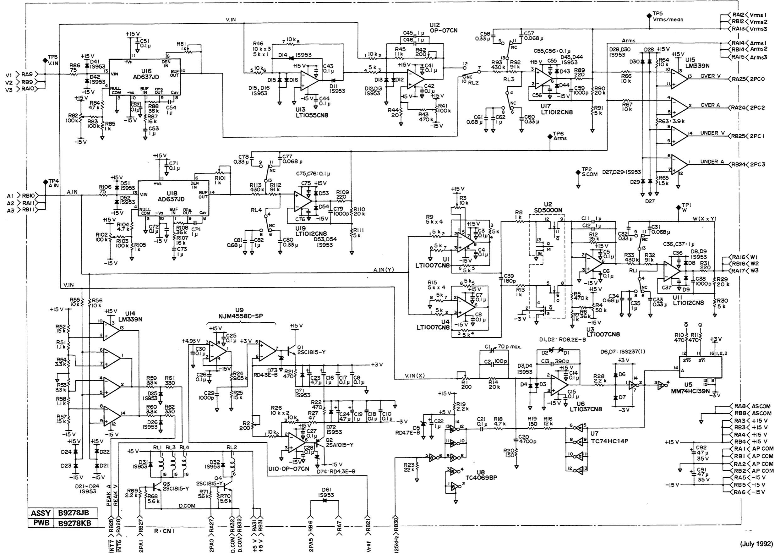
**Figure 5-5a.** RMS Board Ass'y: B9278JB Schematic Diagram.
