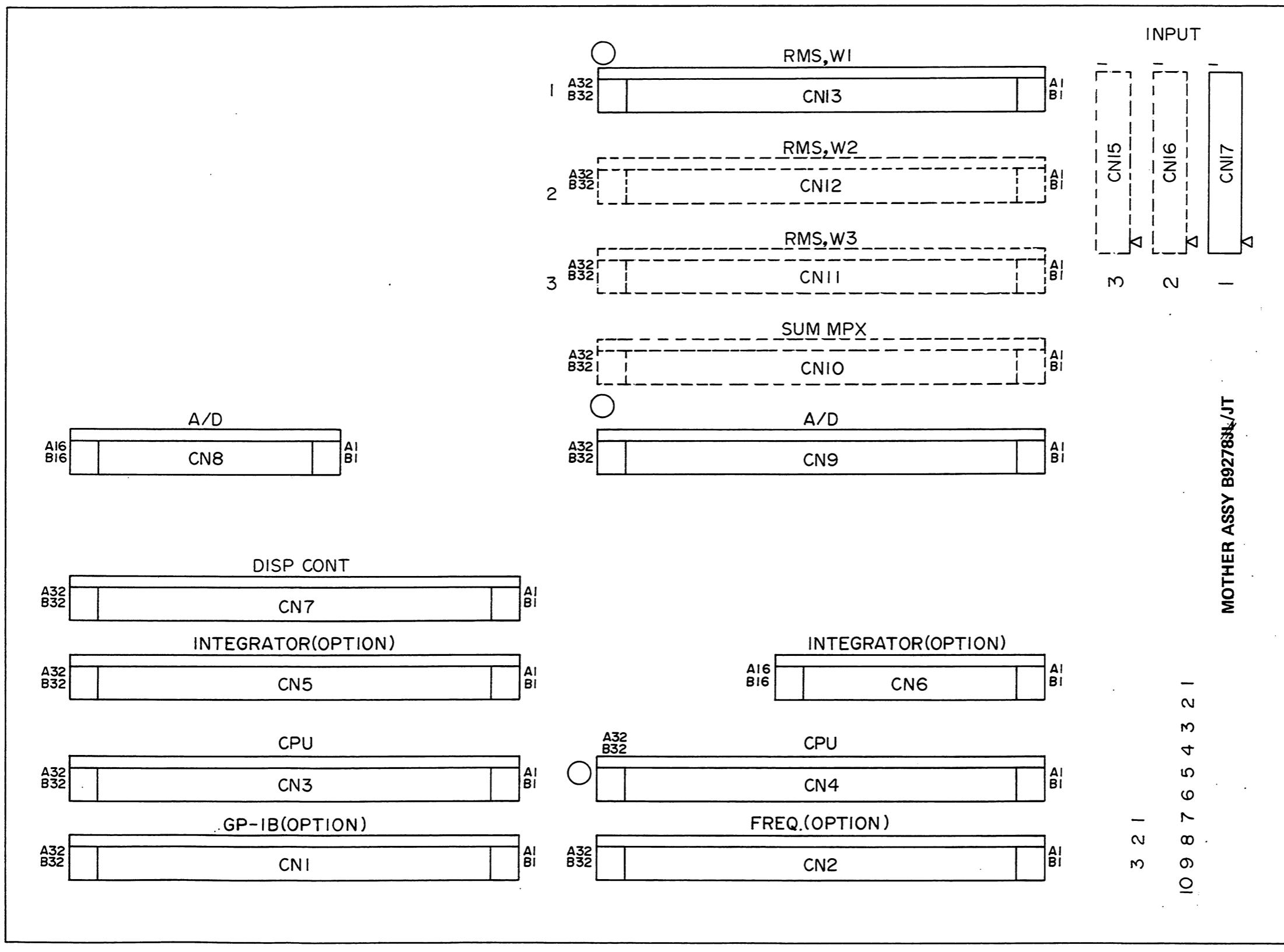
Figure 5-11c. Mother Board Ass'y: B9278JT Components Location Diagram.
