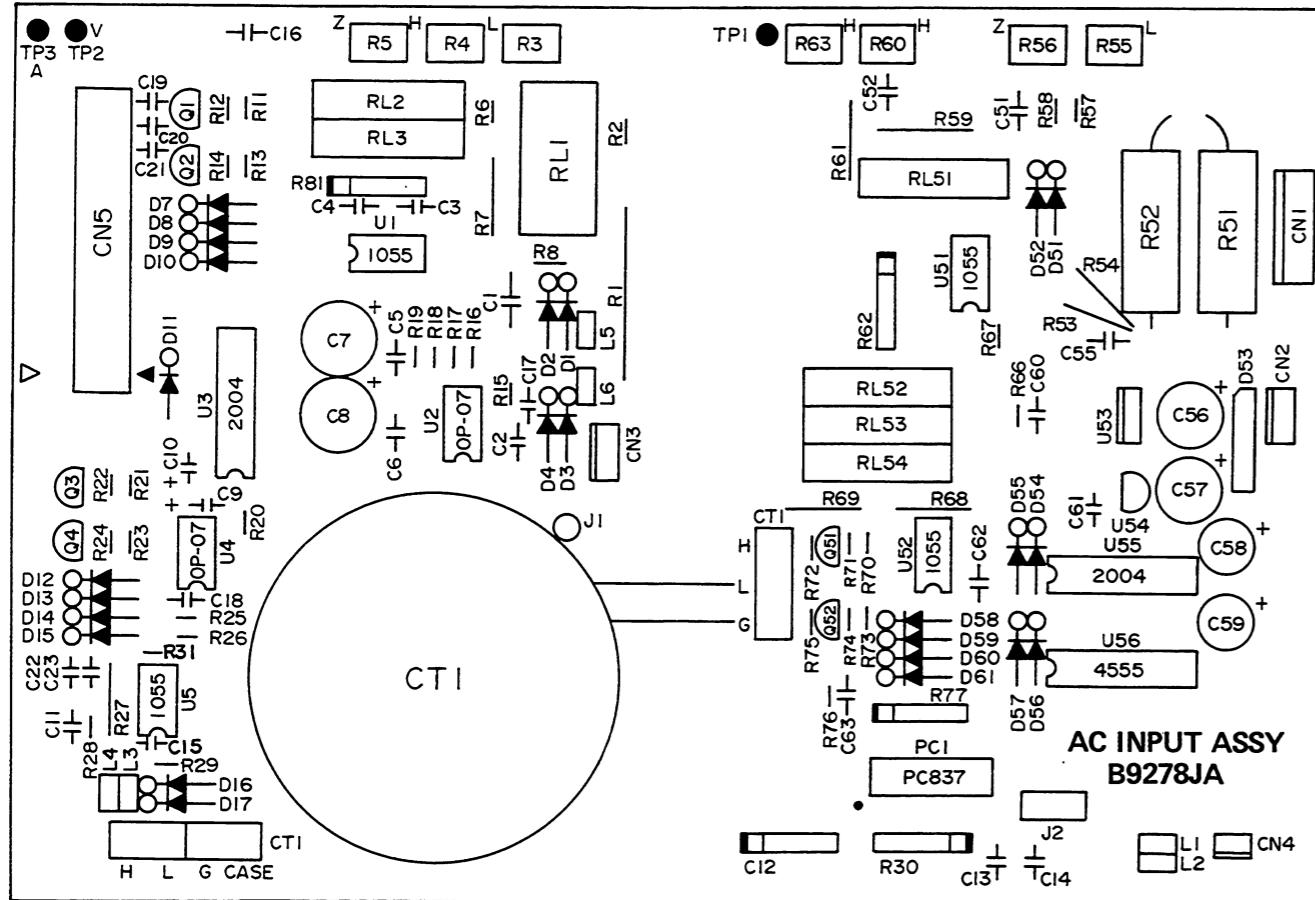
Figure 5-2b. AC Input Board Ass'y (for Model 2533E31): B9278JA Components Location Diagram.
