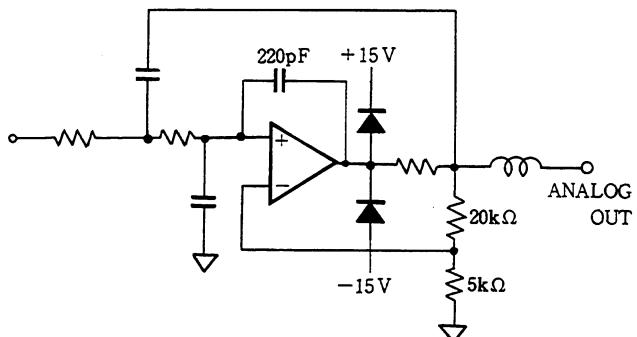
**Figure 2-23. V, A and W Output Circuit**
