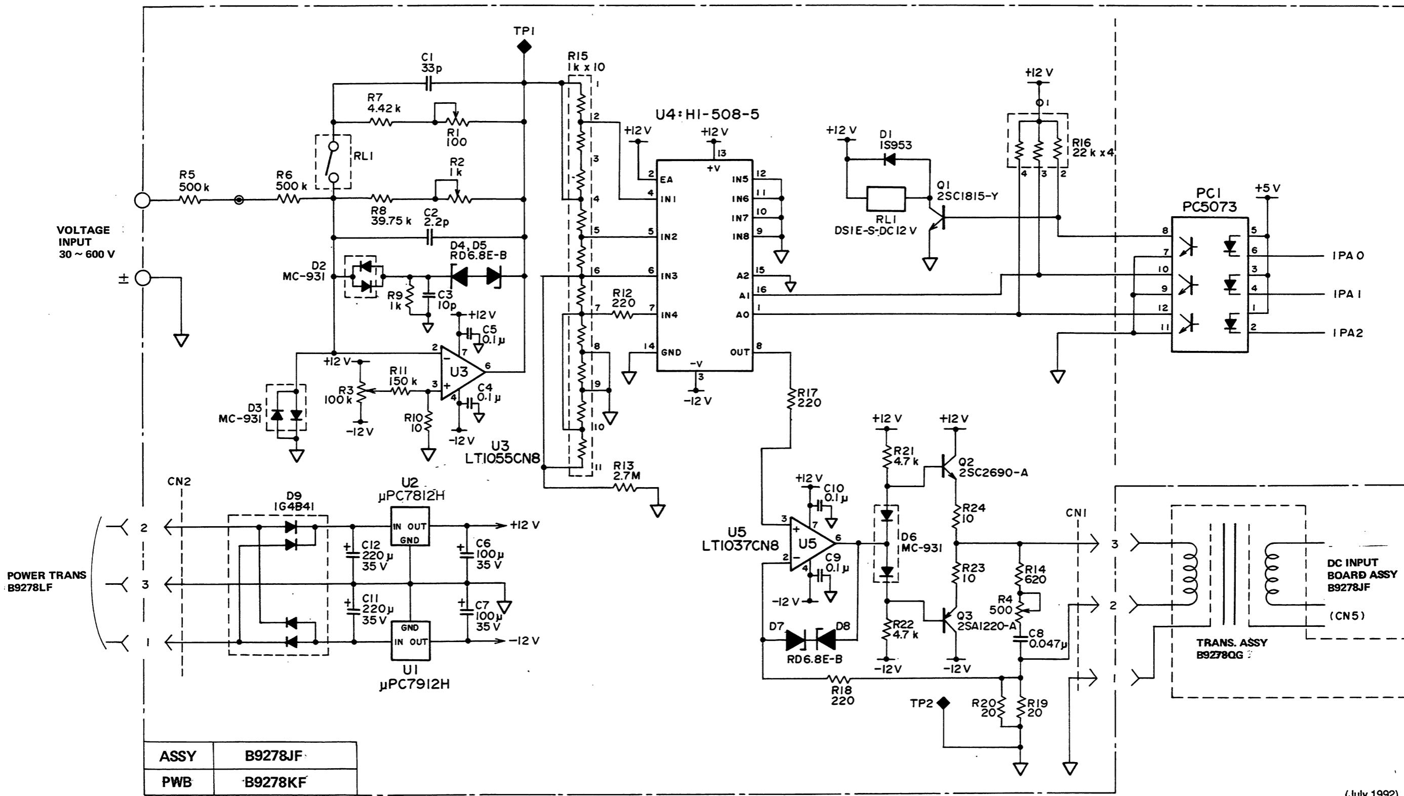
Figure 5-4a. DC Input Board Ass'y (for Model 2533E41): B9278JF Schematic Diagram (1/2).
