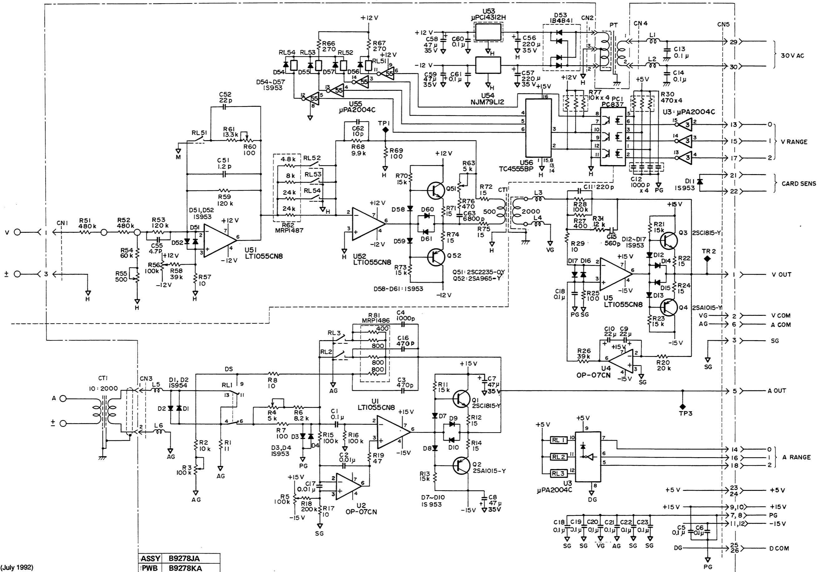
Figure 5-2a. AC Input Board Ass'y (for Model 2533E31): B9278JA Schematic Diagram.
