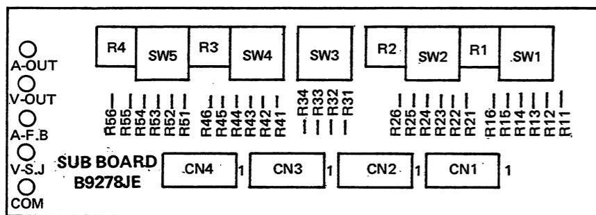
Figure 5-3b. Sub Board Ass'y (for Model 2533E41): B9278JE Components Location Diagram.
