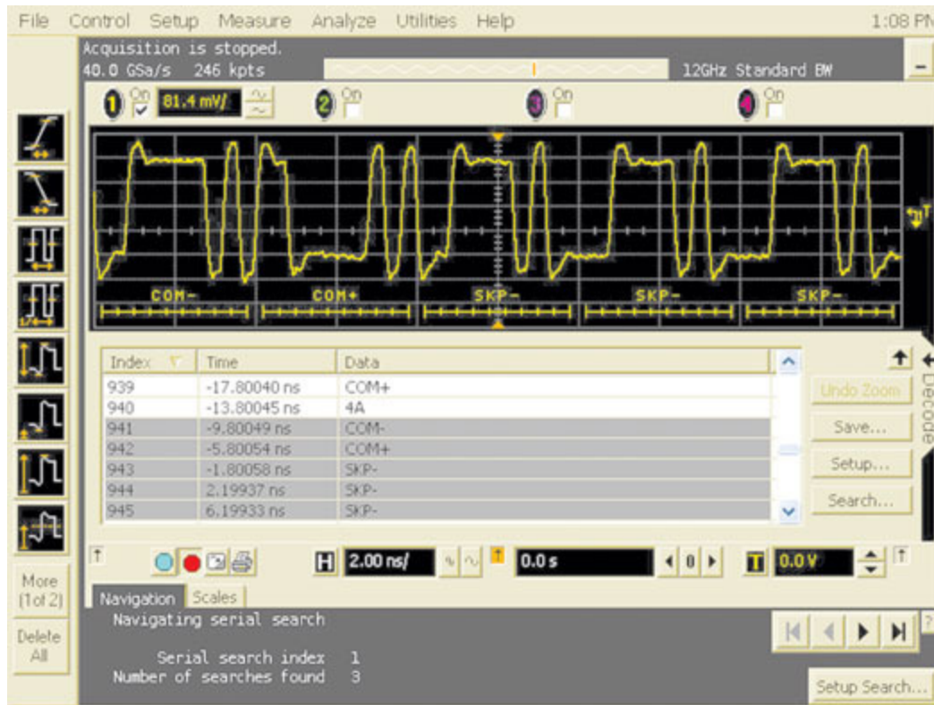
Figure 1. Invalid Character (SKP-) in a PCIe Compliance Pattern Shown Via 8b/10b Decoding
