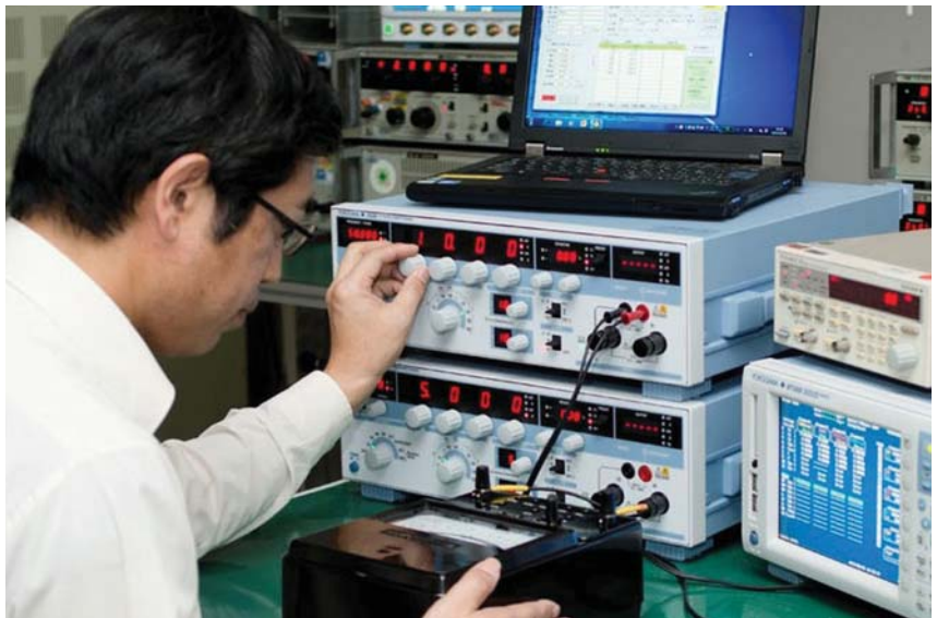
Figure 1: The Yokogawa 2558A is an AC voltage current standard that offers a high accuracy of \pm 0.04\% for AC voltage and \pm 0.05\% for AC current, along with a high stability of \pm 50\text{ppm/h}
