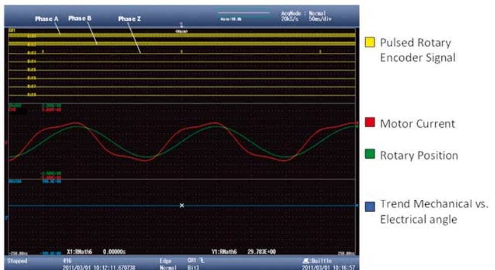
Figure 1. DL850 screen display showing a rotary encoder signal plotted against motor current
