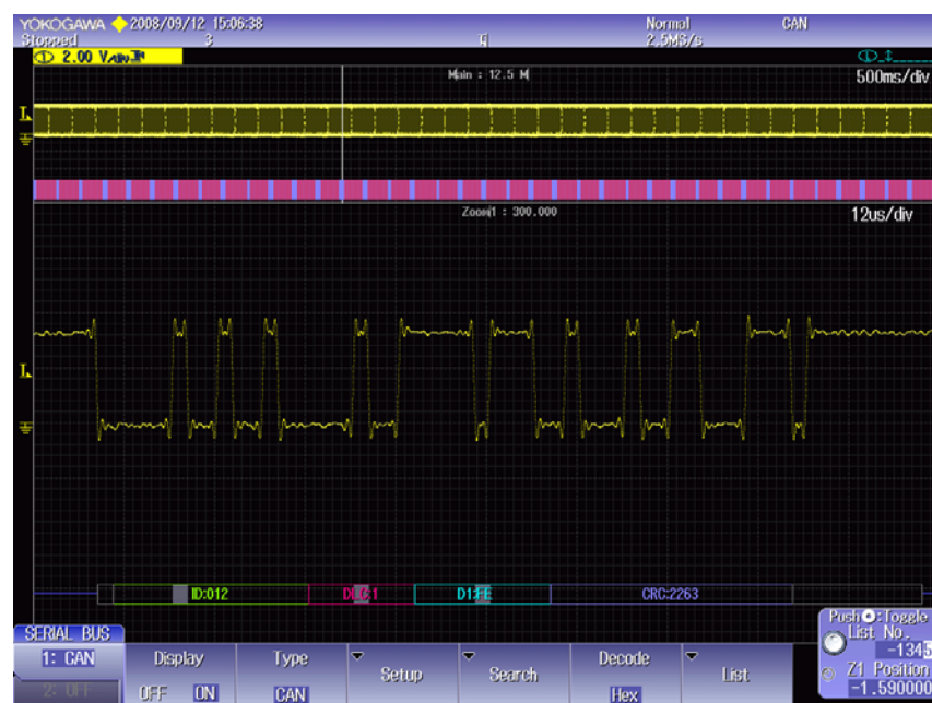
Figure 6 12.5 Mpts CAN waveform (5 sec. duration) and the Zoom window
