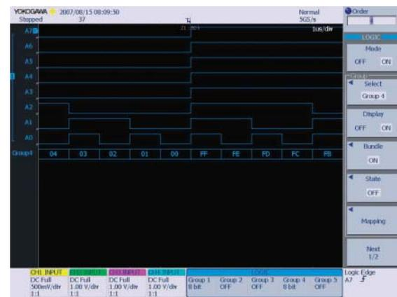
**Figure 5** Bus Display of Grouped Logic Signal
