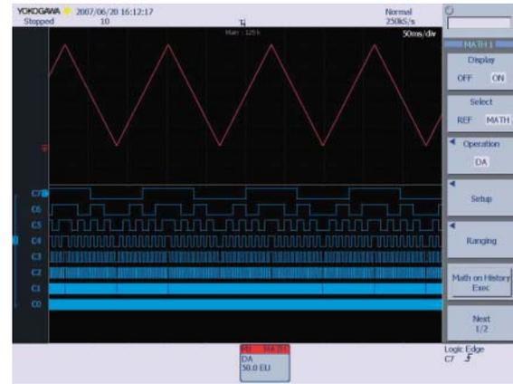
Figure 7 D/A Conversion Display
