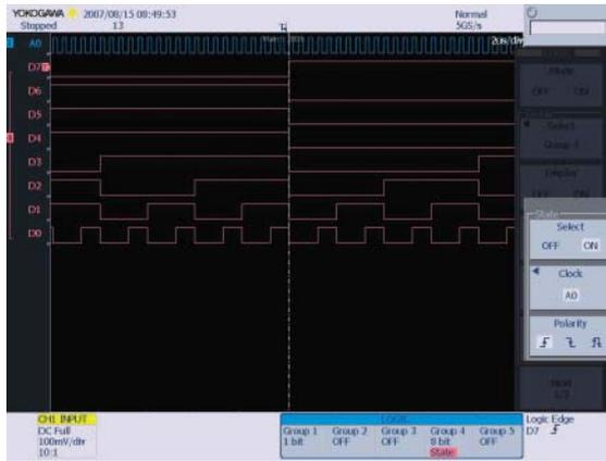
Figure 6 State Display of Logic Signal
