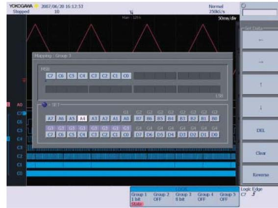
**Figure 4** Logic Signal Grouping Setting Screen
