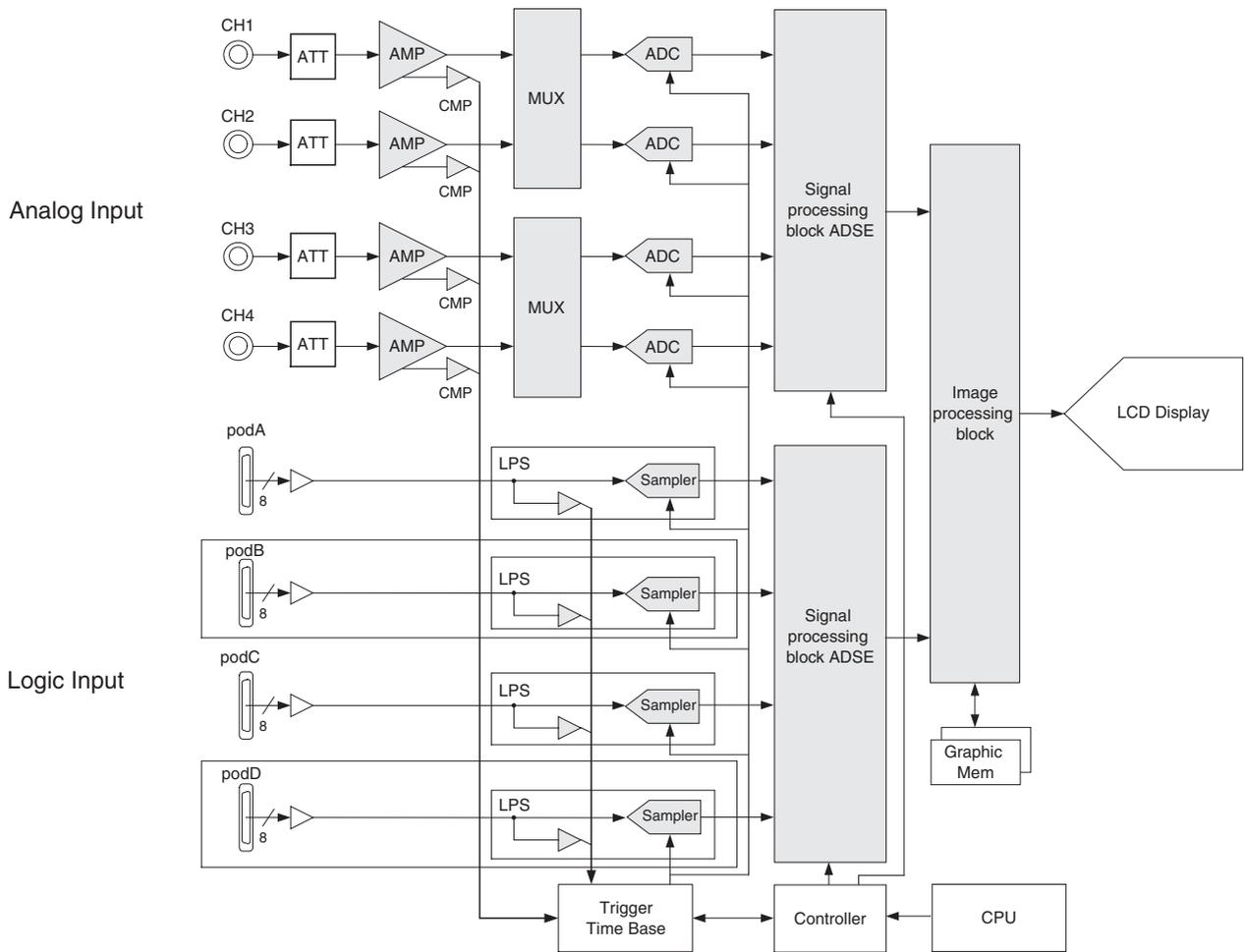
**Figure 2** DL9700/DL9500 Series Configuration (DL9500 is pod A and C only)
