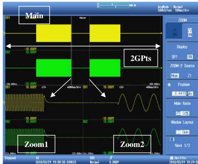
Figure 10 Example of a zoomed waveform
