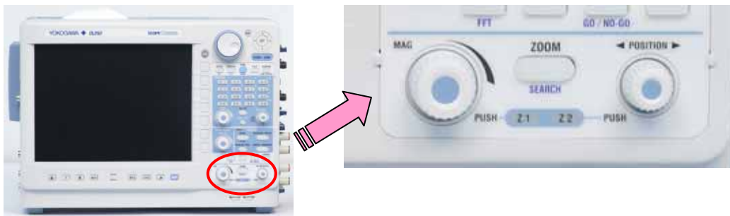
Figure 11 Independent zoom knobs
