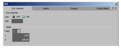
The items in the measurement channel tab and Ext. channel tab can be configured for each channel. The items that are configured are the same as those configured on the spreadsheet. For details, see the page corresponding to the item.
