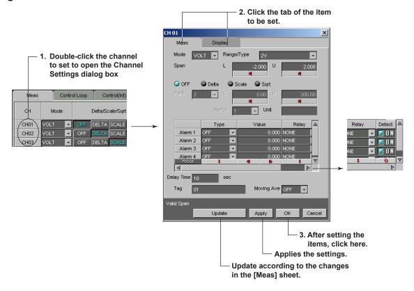
The items of the [Meas] tab can be set for each channel. The items set here are the same as the ones in the [Meas] tab of the Hardware Configurator. For details, see the page corresponding to the item.
