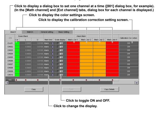
Enter external input channel settings in the same manner as those of the measurement channel items. Also note that this measurement channel setting screen is only one example; your actual screen may vary.
