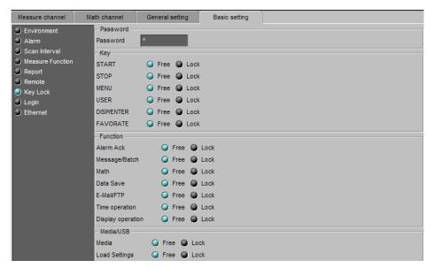
Enabled when [Key Security] is set to [Keylock] under [Environment] - [Detail Setting] in the [Basic Setting] tab. This function is not available on DXs with the /AS1 advanced security option.
