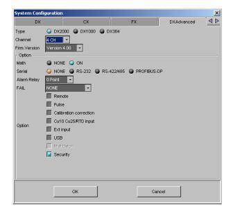
**2.** Configure all the settings on the [DXAdvanced] tab, and then click the [OK] button. The DX1000/DX2000 setting screen in displayed.
