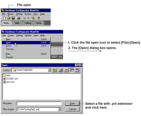
You can specify the location where the setup data file is located and open the Configurator.
