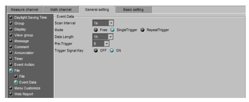
Event related settings are enabled when [Data Kind] is set to [E+D] or [Event] in [Basic Environment] under [Environment] in the [Basic Setting] tab.
