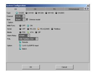
Only the system configuration in the setup data file can be checked. If the system configuration is changed and the [OK] button is clicked, a message "System Configuration is changed Input & Data are Initialized" appears. Clicking the [OK] button initializes the data.
