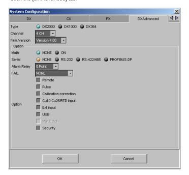
2. Enter all settings on the [DXAdvanced] tab, then click the [OK] button. The DX1000/DX2000 setting screen in displayed.
