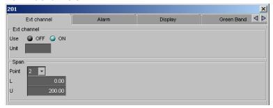
The items in the measurement channel tab and Ext. channel tab can be configured for each channel. The items that are configured are the same as those configured on the spreadsheet. For details, see the page corresponding to the item.
