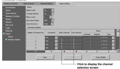
Modbus master settings are enabled when you set [Protocol] to [Master] under [Serial] - [Serial] in the [Basic Setting] tab.
