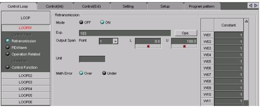
Sets the equation and output span on loops whose control mode is analog retransmission.
