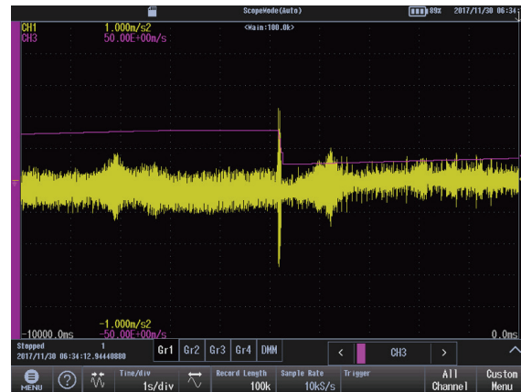
Figure 3 - Velocity data (purple) and vibration data (yellow) showing vibration impulse corresponding to sudden slowdown
