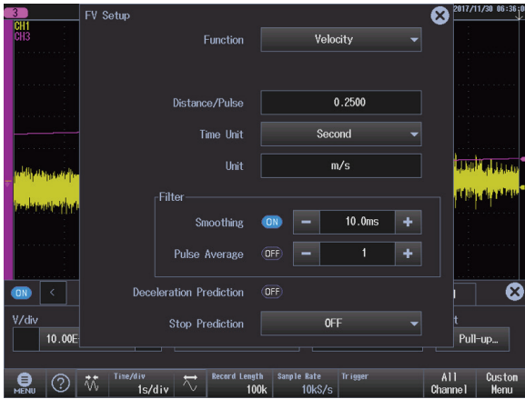
Figure 2 - Velocity setup menu
