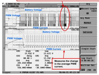
The above figure shows the measured data obtained in an operation test of the ABS control unit. We made the wheels lock up, and measured the influence of battery voltage fluctuations on the PWM current signal.
