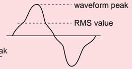
$$\text{Crest factor (CF, peak factor)} = \frac{\text{waveform peak}}{\text{RMS value}}$$
