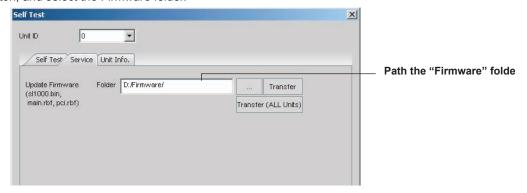
7. Click the Transfer button to execute the firmware version upgrade. During the upgrade, be sure not to turn OFF the power to the main unit. If the version upgrade is successful, the messages in the figure below appears. Turn OFF the power to the main unit, then restart it (if for some reason the restart is not successful, please see the firmware upgrade procedure manual in the Recovery folder).
