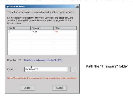
5. Click the Update button. The firmware version upgrade executes. During the upgrade, be sure not to turn OFF the power to the main unit. If the version upgrade is successful, the state changes to OK, and the message in the figure is displayed. Turn OFF the power to the main unit, then restart it (if for some reason the restart is not successful, please see the firmware upgrade user's manual in the Recovery folder).
