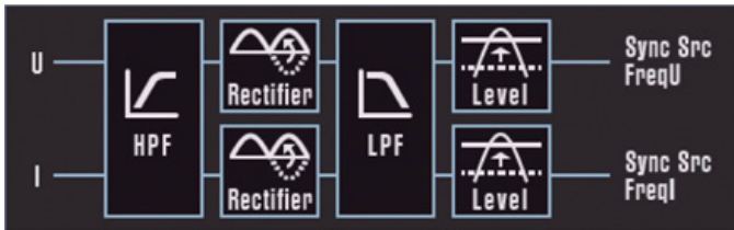
Figure 6. Filters can apply anti-alias filters and digital line filters on normal measurements and harmonic measurements.
