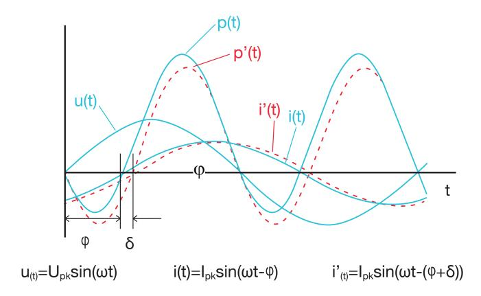
While this has no effect on rms voltage or current or apparent power measurements, it does influence the measurement of active power and hence also the power factor. This phase shift should be specified by power analyzer manufacturers to account for all boundary conditions that can affect phase angle error and other measurement errors.
