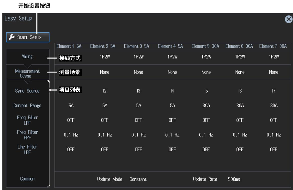
The screenshot shows the 'Easy Setup' interface with the 'Wiring' section selected. The main area displays a table for setting up seven elements (Element 1 to Element 7) with various parameters like current range, filter settings, and update modes.
