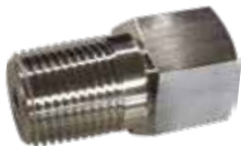
接头91086 (1/2" NPT公接头转1/4" NPT母接头)
