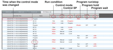
The name of the loop in which the control mode changed or whether or not the mode change was due to program control
