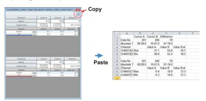
When cursor values are copied from the cursor value dialog box, the data is copied with a row inserted between Waveform1 and Waveform2 as shown in the figure.
