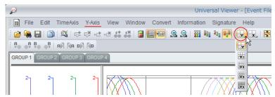
Select a density from the **Y-Axis** menu, or click the corresponding button on the toolbar. To change the density of the grid lines on the time axis (X-axis), select a density from the **TimeAxis** menu, or click the corresponding button on the toolbar. You can select the grid line density from five levels.
