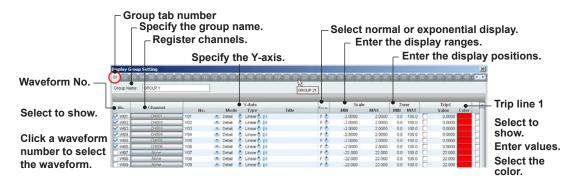
Specify the Y-axis grid line spacing. Leave unselected to use the default grid line spacing. To specify the grid line spacing, select the check box and enter a value.
