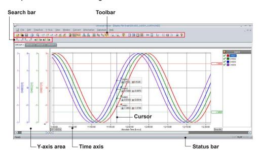
The commands that correspond to the buttons on the toolbar, search bar, and superimposed display toolbar are described on the subsequent pages. The buttons on the toolbar correspond to the commands in the menus. If the window does not have certain menus, the corresponding buttons on the toolbar are disabled.
