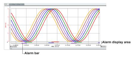
Alarm bars are displayed in order from the top: alarm 1, alarm 2, alarm 3, and alarm 4. When alarm bars overlap, alarm bars are displayed from the front with the following precedence: the active waveform, waveforms with the same Y-axis as the active waveform, and waveforms in the same display group with smaller waveform numbers.
