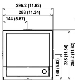
(Dimensions before attaching the mounting bracket)
