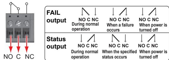
Recommended torque for tightening the screws: 0.5N•m
