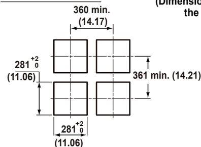
(Dimensions after attaching the mounting bracket)
