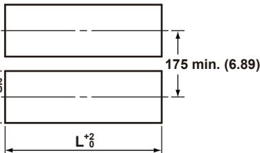
**Side-by side mounting (vertically; max. 3 units)**
