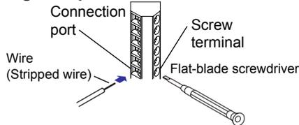
First, loosen the screw at the front using a flat-blade screwdriver. Insert the input signal wire into the slit on the left side of the terminal block, and fasten the screw at the front.
