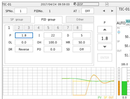
**5 Tap ▲ or ▼ to change the value. To confirm the value, tap ENTER. You can also enter the value directly from the keyboard by tapping the center value.**
