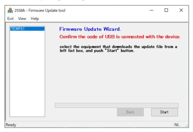
6. A progress bar shows the progress.Do not remove the USB cable or turn off the 2558A until updating is finished.
