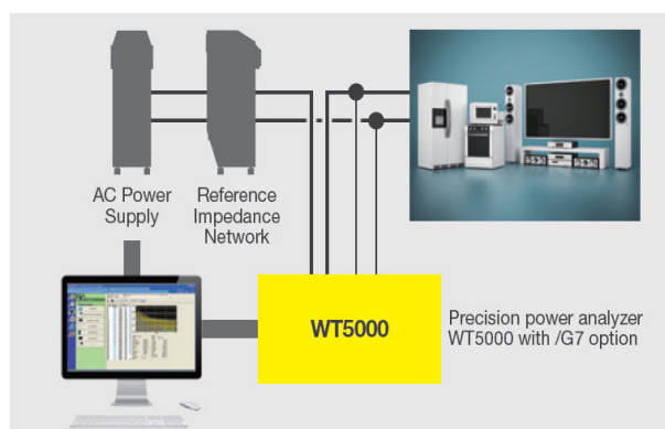
Figure 7. System example and display of harmonic measurement, report example
