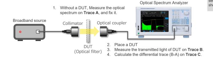
The smaller the numerical aperture (NA) of the optical fiber and the shorter the optical path length from the collimator to the optical coupler, the smaller the loss, which is advantageous for measurement, but high precision adjustment of angle and optical axis is required. Especially the adjustment of the optical coupler side becomes difficult. Therefore, when the optical power is high, it is easier to adjust it by receiving light directly with the ferrule of the optical fiber.
