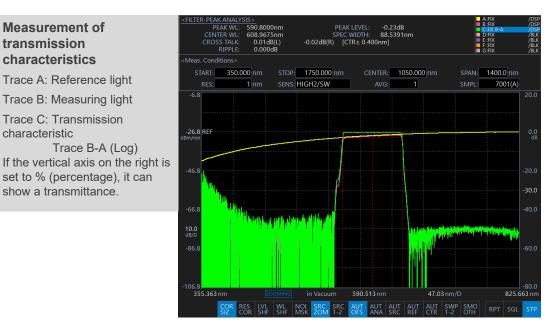
AN OSA-Measurement of transmission characteristics of optical filter-EN
