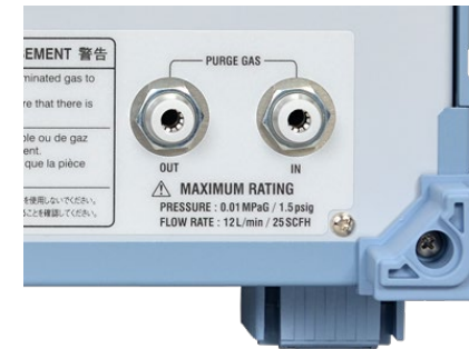
Purging gas ports (IN/OUT)
