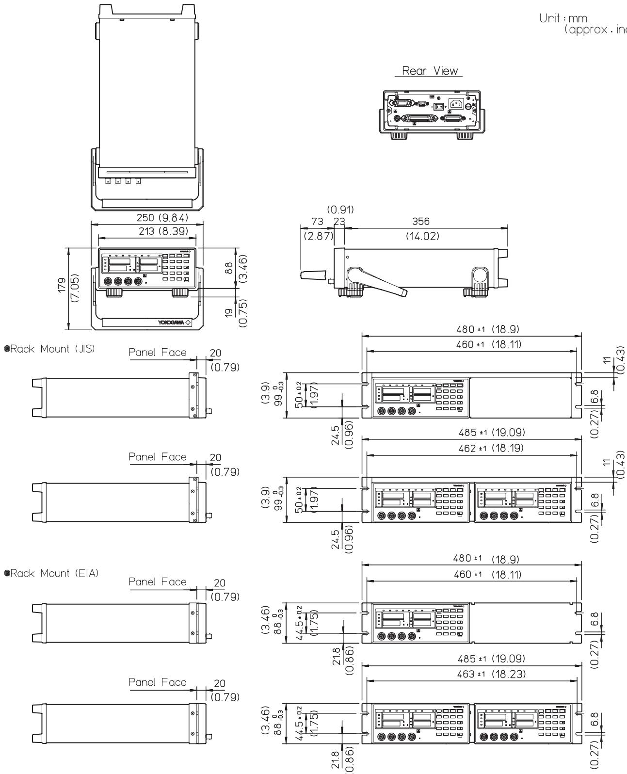
If not specified, the tolerance is  $\pm 3\%$ . However, in cases of less than 10mm, the tolerance is  $\pm 0.3\text{mm}$ .
