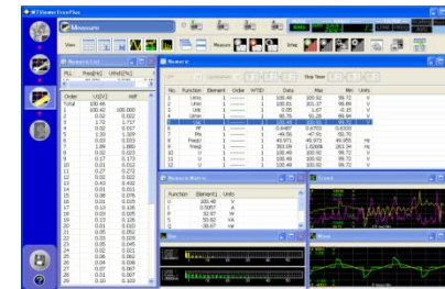
■ WTVIEWERFreePlus Screen (Measurement is started by simply clicking the "▲" at the top of the screen.)
