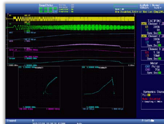
Example of waveform display and evaluation of I-T and S-T characteristics
