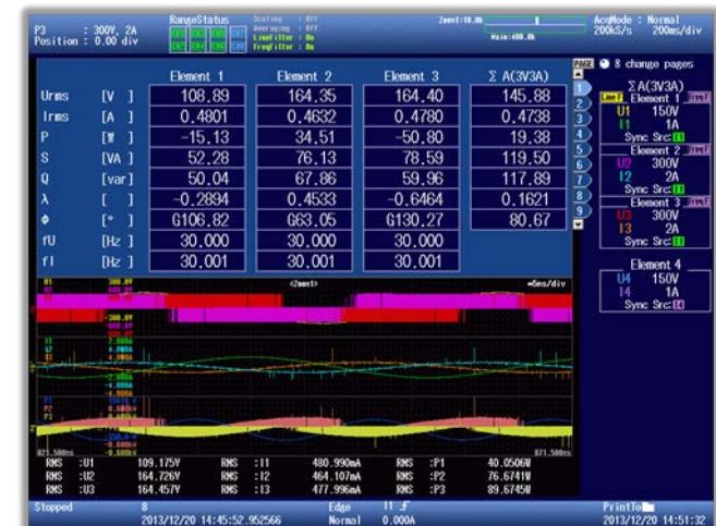
Measures inverter waveform at 100 MS/s and displays voltage, current, power results.
