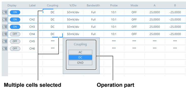
2. Change the setting information. Cells with the setting information the same as that of the first clicked cell are changed at a time. Cells with the setting information different from that of the first clicked cell are not changed.
