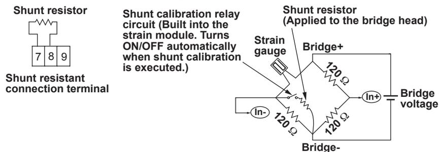
For specific instructions on performing shunt calibration, refer to your measuring instrument's user's manual. For information on shunt resistance and the corresponding strain values, see page 13 in "Calculation of the Shunt Resistance."
