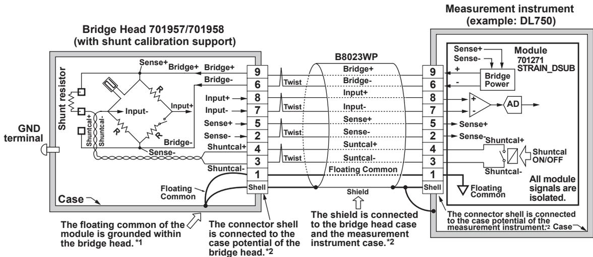
\*1 The GND (floating common) of the module is connected to the case potential inside the bridge head.
