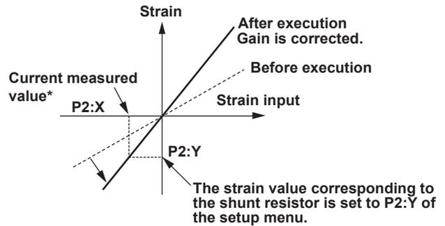
\* Automatically obtained when shunt calibration is executed.
