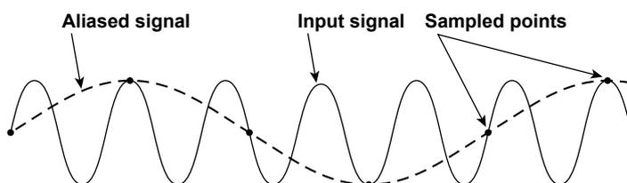
Aliasing causes problems such as increased errors in measured values and incorrect measurements of the phase angles on each harmonic. An anti-aliasing filter is used to prevent aliasing and eliminate high frequency components that are irrelevant to the harmonic measurement.
