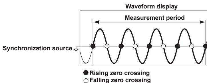
If there is not more than one rising or falling slope within the waveform display, the entire waveform display is set as the measurement period.
