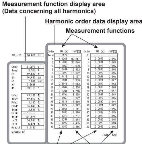
**Numeric data for each harmonic**      **Distortion factors of each harmonic (When the selected measurement function is U, I, or P, Uhdf, Ihdf, or Phdf is displayed.)**
