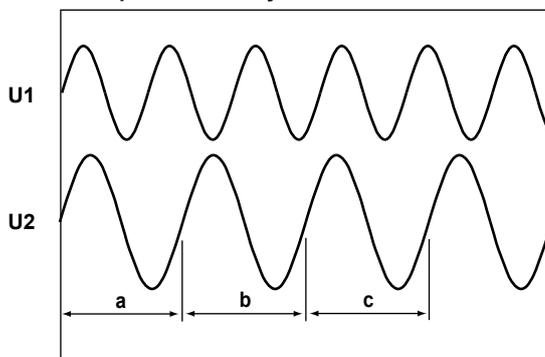
Measures the items in ranges a, b, and c, and calculates statistics on the items in the order a, b, and c.
