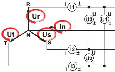
\* In the measurement functions, *rms*, *mn(mean)*, *dc*, *rmn(r-mean)*, and *ac* are the delta computation modes. A indicates the wiring unit.
