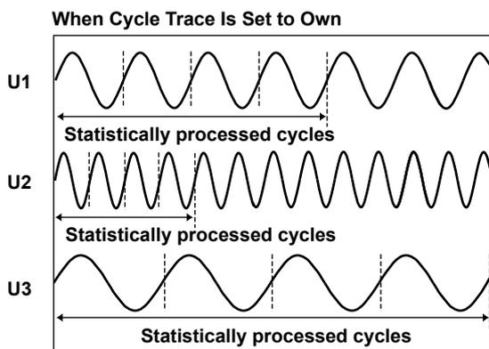
The number of cycles in the channel with the slowest cycle (U3) is four, so statistical processing is performed on the four oldest cycles of the data for U1 and U2. The remaining data is not used for statistical processing.
