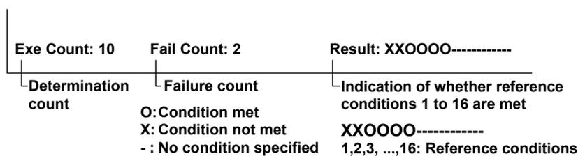
In this example, reference conditions 1 and 2 are not met while the conditions defined by base waveforms 3 to 6 are met.
