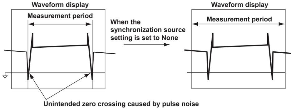
**Setting the Synchronization Period When Measuring a Three-Phase Device**
