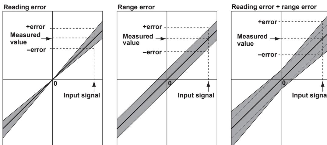
To see how much error is included in the measured values, let us look at several computation examples for a 60 Hz sine wave input signal.
