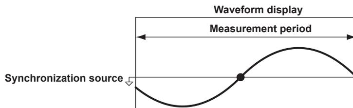
Because of the reasons described above, the measured voltage and current values may be unstable. If this happens, lengthen the time axis setting (TIME/DIV) so that more periods of the input signal fit within the waveform display.
