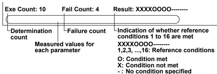
In this example, reference conditions 1 and 4 are not met while reference conditions 5 to 8 are met.
