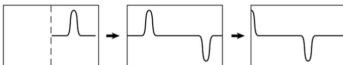
This allows waveforms to be observed in the same way as on a pen recorder. Roll mode is useful for observing signals with long repeating periods and signals that change slowly. It is also effective when you want to detect occasional glitches (pulse signals in the waveform).
