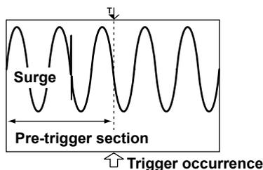
When you use the wave window trigger, we recommend that you set a pre-trigger length that is longer than the reference cycle so that you can observe waveform abnormalities that occur in the reference cycle.
