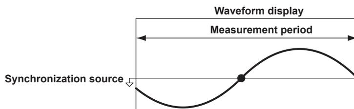
The measurement period for determining the numeric data of the peak voltage or peak current is always the entire waveform display. Therefore, the measurement period for the measurement functions that are determined on the basis of the maximum voltage or current value (U+pk, U-pk, I+pk, I-pk, CfU, and Cfl) is also the entire waveform display.
