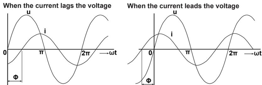
A vector display is used to clearly convey the magnitude and phase relationships between the voltage and current. A positive phase angle is represented by a counterclockwise angle with respect to the vertical axis. Normally, a dot is placed above the symbol representing a quantity to explicitly indicate that it is a vector. The magnitude of a vector represents the rms value.
