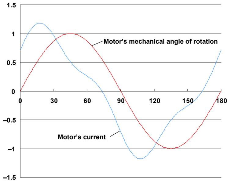
The phase difference is calculated with the motor's mechanical angle of rotation as the reference. If the phase is leading the motor's mechanical angle of rotation, the phase is displayed as a positive value.
