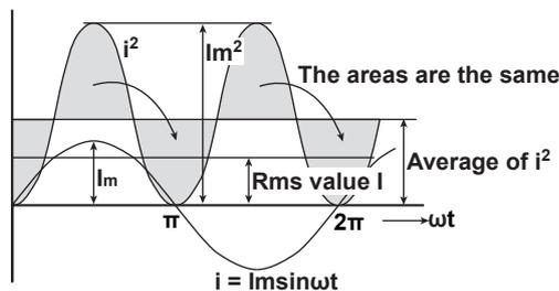
The rms value (effective value) is the DC value that generates the same thermal action as the alternating current. With  $I$  as the DC value that produces the same thermal action as the alternating current:
