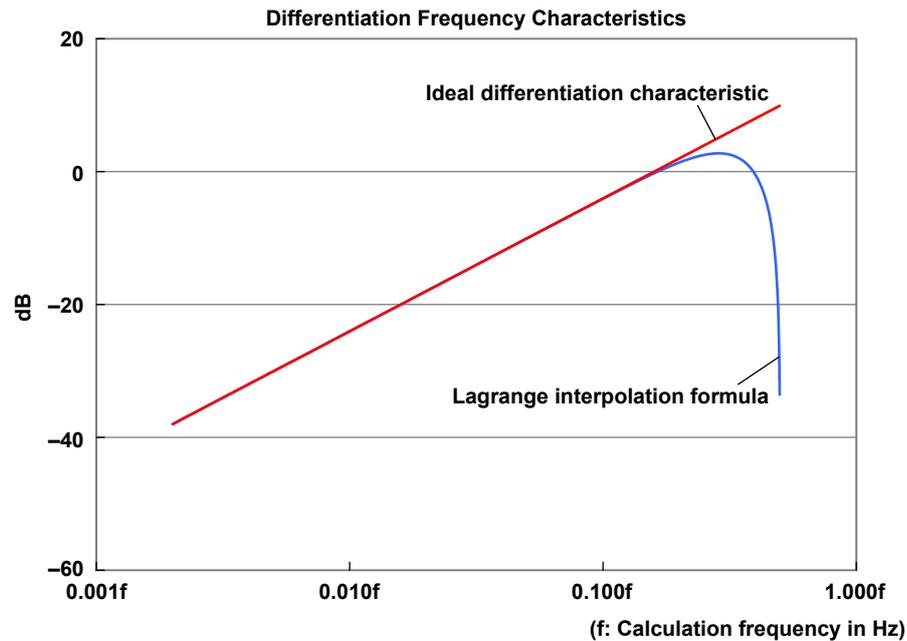
Up to the point where the input frequency is 20% of the calculation period, the differentiation characteristic is almost the same as the ideal differentiation characteristic. At higher frequencies, the high frequency components are restrained by the high-area characteristics of the Lagrange interpolation formula.
