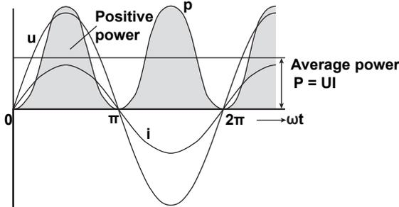
When the phase difference between voltage and current is  $\Phi$
