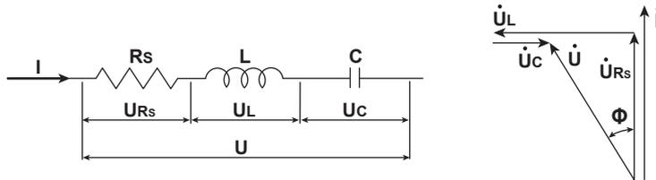
The relationship between resistance  $R_S$ , reactance  $X_S$ , and impedance  $Z$  is expressed by the equations below.
