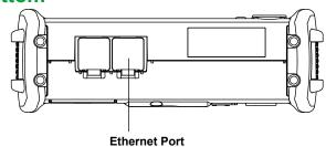
Connector used to connect the AQ1100 to the controller (such as a PC) using a ethernet cable.
