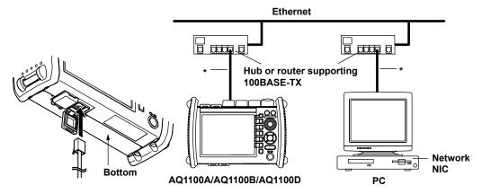
\* UTP cable or STP cable (straight cable in either case)
