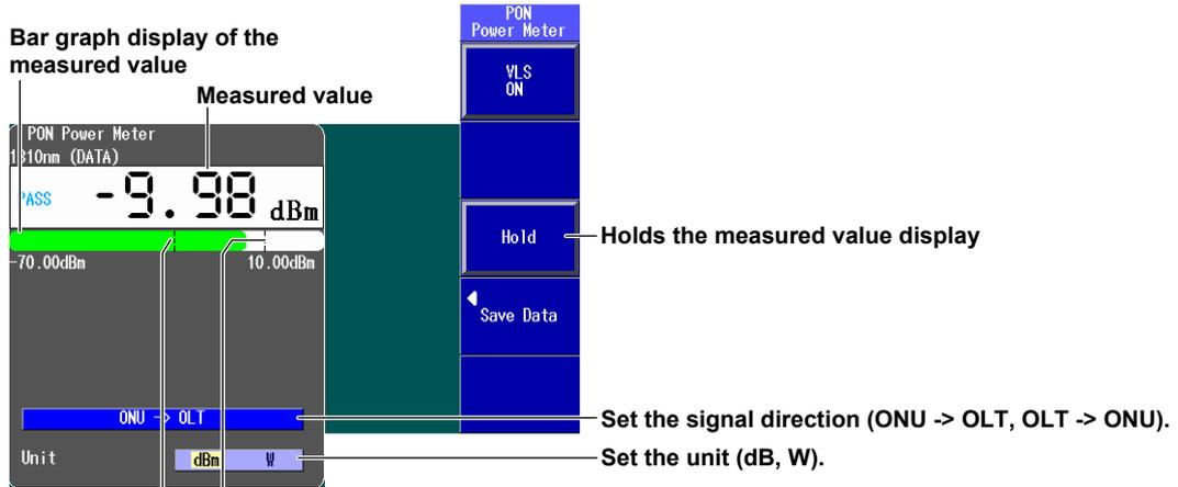
Lower threshold line Upper threshold line
