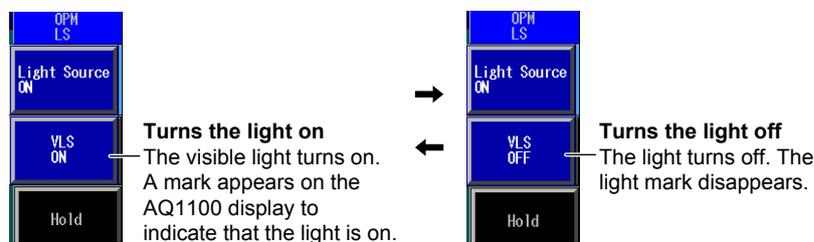
While the above menu is displayed, you can also turn the light on and off by pressing **VLS**.
