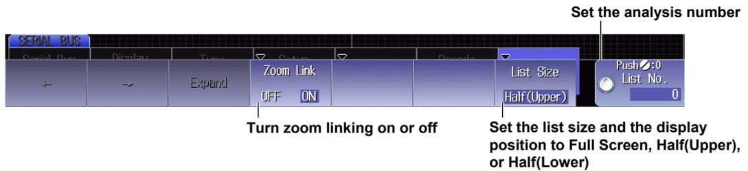
Data before the trigger position (on the left side of the waveform display) is assigned analysis numbers in descending order (-1, -2, and so on). Data after the trigger position (on the right side of the waveform display) is assigned analysis numbers in ascending order (0, 1, 2, and so on).
