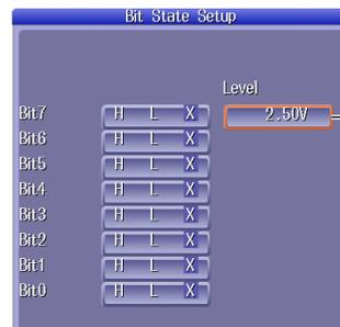
Set the level used to detect each signal's slope, H, L, IN, and OUT states
