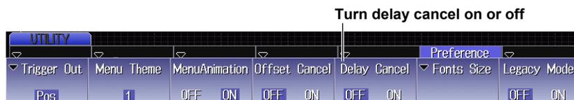
You can select whether or not to apply the specified trigger delay to the time measurement values.
