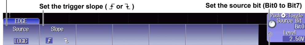
Set the source bit trigger level
