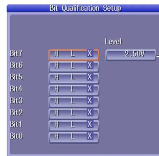
Set the level used to detect each signal's slope, H, L, IN, and OUT states
