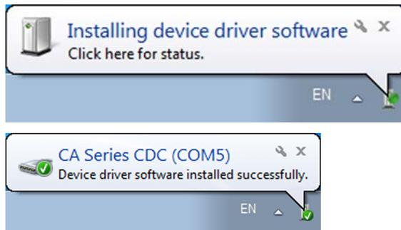
When the driver has been successfully installed, “CA Series CDC” appears in the list of Ports (COM & LPT) in the Device Manager.
