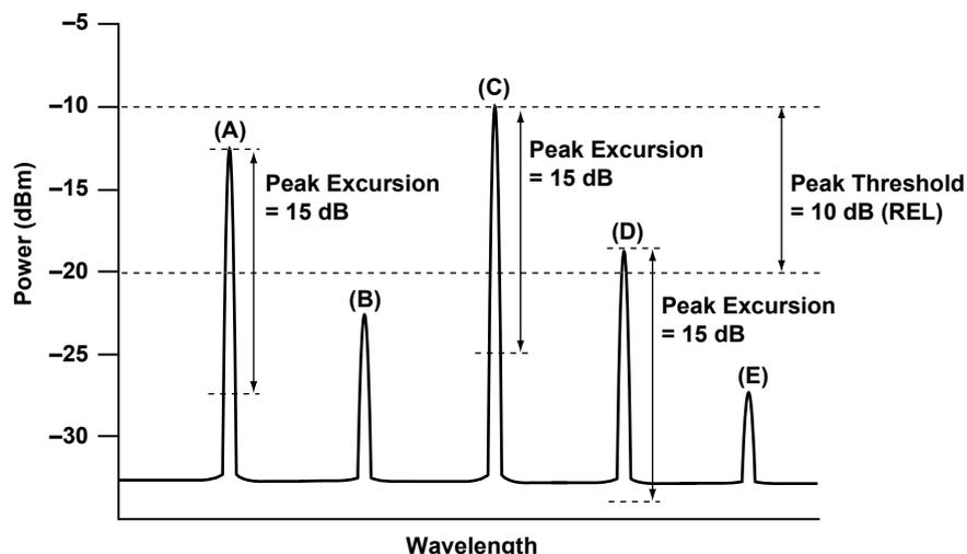
In the above example, only (A) and (C) are detected as peaks.
