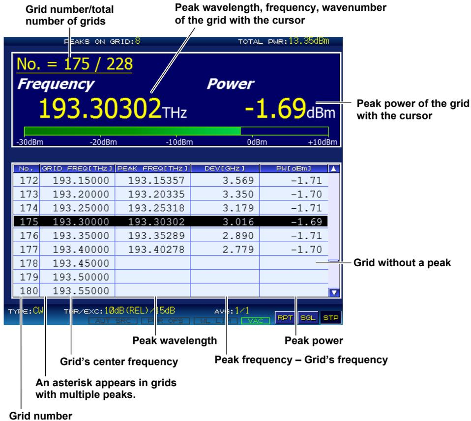
The list displays grid numbers, grid frequencies (wavelength, wavenumber), peak frequency (wavelength, wavenumber), frequency deviation (wavelength difference, wavenumber difference) of the grids and peaks, and peak power.
