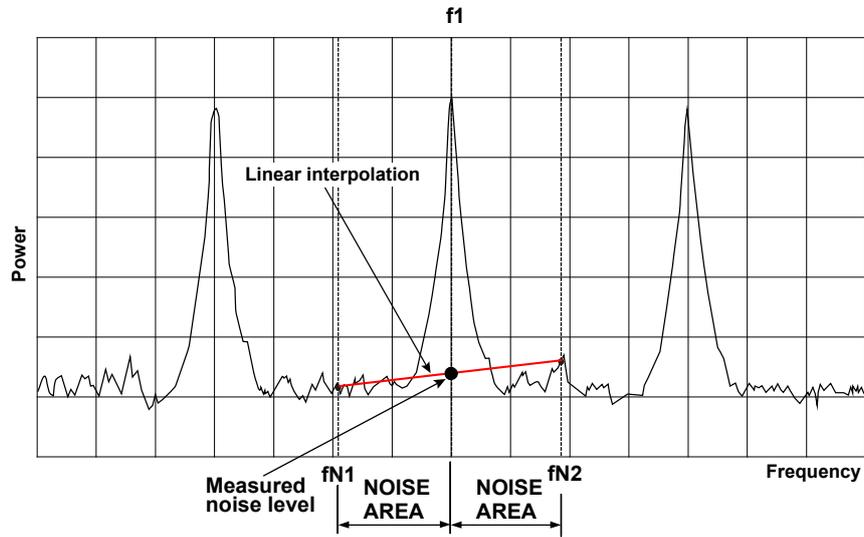
NOISE AREA can be set automatically or manually according to the NOISE ALGO setting.
