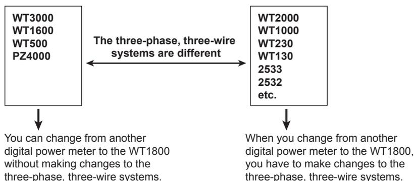
For example, if you replace the WT1000 (used in a three-phase, three-wire system) with the WT1800 and leave the wiring unchanged, the measured power of each element will be different between the WT1000 and the WT1800. Refer to this manual and re-wire the system correctly.
