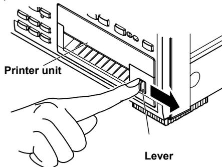
2. Insert your finger into the groove on the right side of the printer unit.
