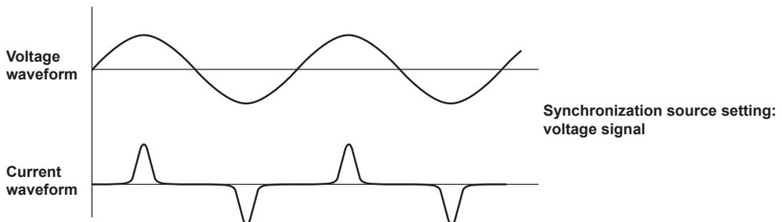
As another example, if an inverter is being measured and the current waveform distortion is smaller than the voltage waveform distortion, set the synchronization source to the current signal.
