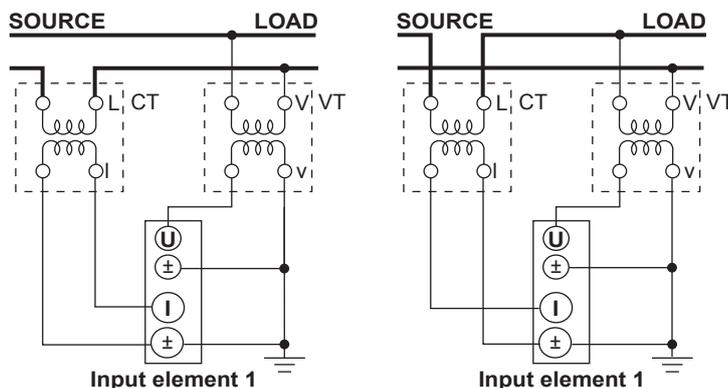
**Wiring Example of a Single-Phase, Three-Wire System (1P3W) with VTs and CTs**
