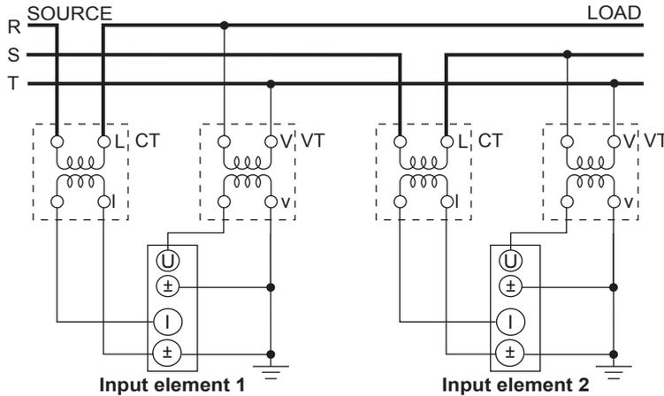
**Wiring Example of a Three-Phase, Three-Wire System That Uses a Three-Voltage, Three-Current Method (3P3W; 3V3A) with VTs and CTs**
