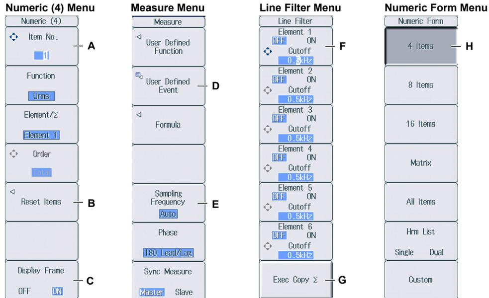
A: Press the soft key to use the cursor keys to configure this setting. Use the cursor keys to set the value or select an item.
