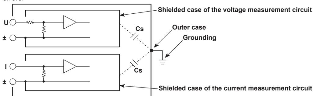
As an example, we will consider the case when the outer case and one side of the power supply are grounded.
