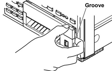
3. Hold the top, bottom, and right side of the printer unit, and then pull it toward you until it stops (pull the unit approximately 5 cm).
