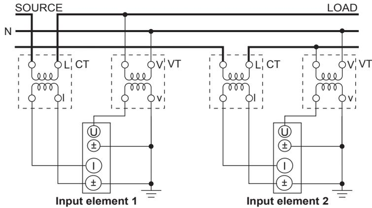
**Wiring Example of a Three-Phase, Three-Wire System (3P3W) with VTs and CTs**
