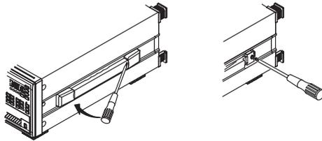
2. Remove the four feet from the bottom of the instrument.
