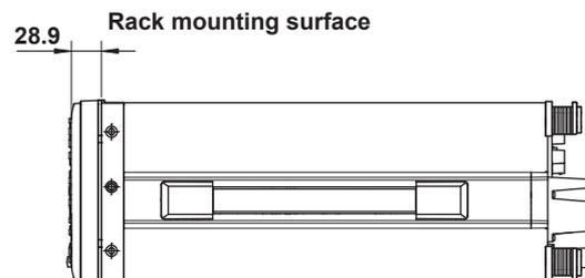
Unless otherwise specified, tolerances are ±3% (however, tolerances are ±0.3 mm when below 10 mm).
