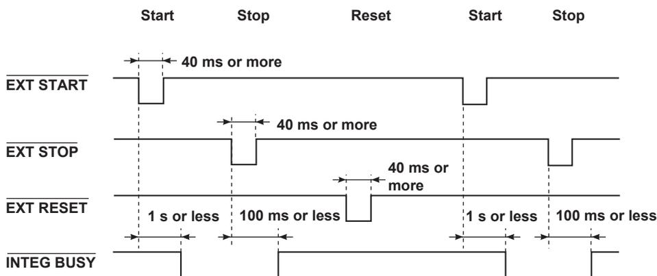
The **INTEG BUSY** output signal is set to low level during integration. Use this signal when you are observing integration.
