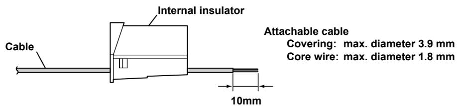
2. Insert the tip of the cable into the plug. Fasten the cable in place using the hexagonal wrench.
