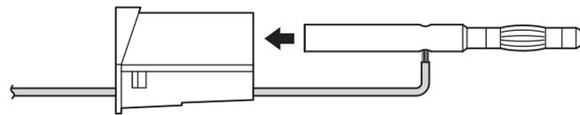
4. Attach the external cover. Make sure that the cover does not come off.
