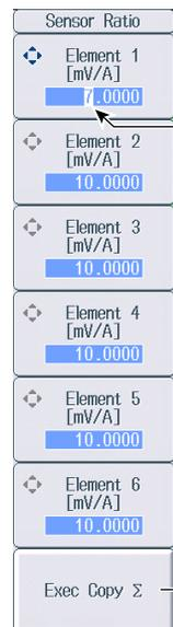
The screenshot shows a menu titled "Sensor Ratio" with six elements, each labeled "Element 1" through "Element 6" with a unit of "[mV/A]". Below each element is a blue bar displaying a conversion ratio. Element 1 shows "7.0000", while Elements 2 through 6 show "10.0000". At the bottom of the menu is an option labeled "Exec Copy Σ".
