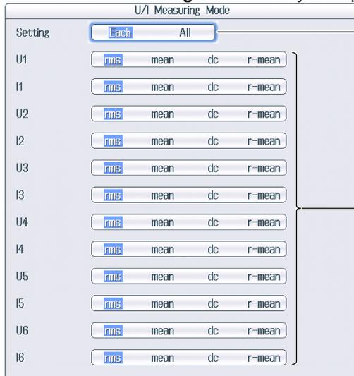
**Select the measurement mode setup method (Each, All).**
