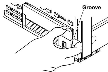
3. Hold the top, bottom, and right side of the printer unit, and then pull it toward you until it stops (pull the unit approximately 5 cm).
