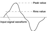
On this instrument, the crest factor is the ratio of the maximum applicable peak value to the measurement range.
