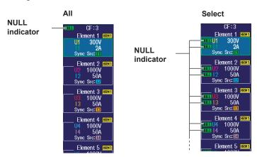
If you press NULL while the NULL feature is enabled, the NULL key light and NULL indicators turn off, and the NULL feature is disabled.
