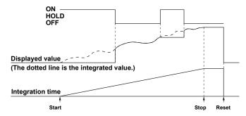
• If you stop integration while the display is held, the displayed and transmitted values do not change. When you release the hold function (turn it off) or make a single measurement by pressing SINGLE, the integration result at the point when integration was stopped is displayed and transmitted.
