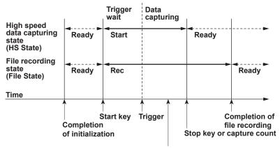
After a trigger occurs, measured data is regularly written to the high speed data capturing data file (.WTS).
