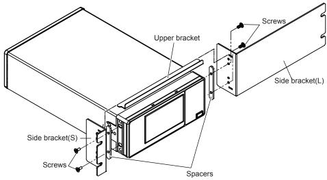
The above figure is an example of mounting the measuring instrument toward the left side. You can mount the measuring instrument toward the right side by interchanging the small side bracket and the large side bracket.
